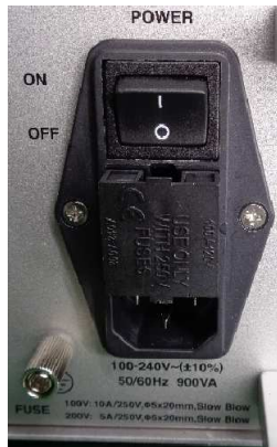
④ State the fuse holder is pulled out
