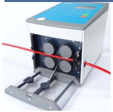
Cross cutting Machine only for tubes up to 8 mm (0.32") outer diameter. Straight cut surfaces thanks to the use of special tube guides.
