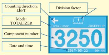
**2) PRESET MODE:** the desired component number is keyed on the keyboard and the counter automatically stops when it reaches the corresponding component
