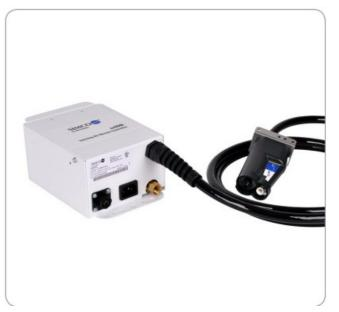
The orION features high blow-off force capability combined with fast removal of electrostatic surface charge. Reliable balance stability is maintained at better than  $\pm 15V$ . An easily replaceable 0.01-micron particle filter is positioned at the nozzle air exit to provide the highest confidence that clean air is delivered to sensitive product.
