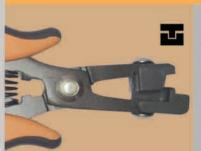
PN 5050/4 Special tool for the forming of side leads of TO 247 with 5.08mm pitch.
