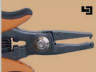
Specially designed tool for end cutting, suitable for access in dense areas of PCBs. It cuts and bends the component lead in one operation, fixing it to the circuit board.
