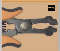
Specially designed tool for pre-forming and cutting of IC pins in one operation.
