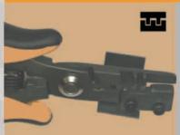
Special tool that enables TO220 component leads (5 leads) to be bent at a 90°angle in a single operation, in such a way that 1- 3 - 5 leads will be 2.54 mm shorter than 2 - 4 leads.
