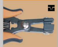
Specially designed tool for the forming of centre lead of TO 247 and TO 220 with 5.08mm pitch. Dissipative version available.
