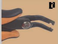
A specially designed forming tool that C shapes the component wire. Bent at 45°.
