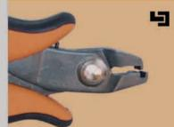
A special tool that cuts and bends the component wire against the PCB in one operation.
