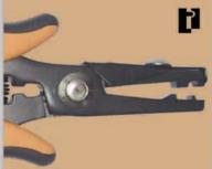
A special tool that cuts and forms the component wire in one operation. Lenght setting is carried out by means of a sliding stop (A min 3 max 16).
