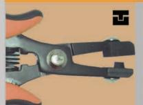
PN 5050/15 Specially designed tool for the forming of centre lead of TO 220 with 2.5mm pitch. Dissipative version available.
